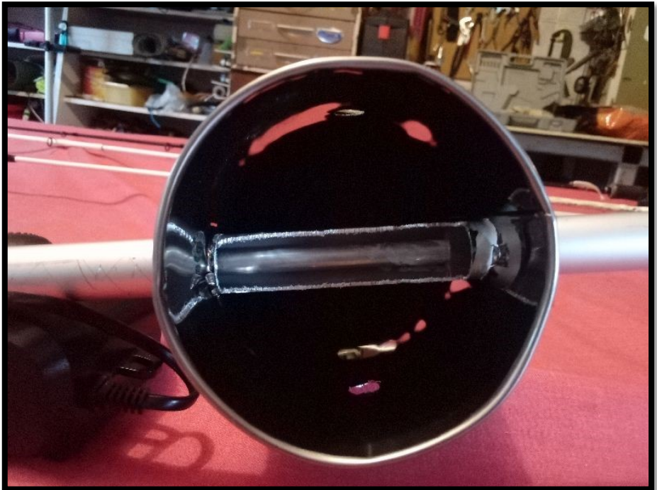
A venturi inside the chamber which keeps the wood chips smouldering. Photo: Roger Bowden.
